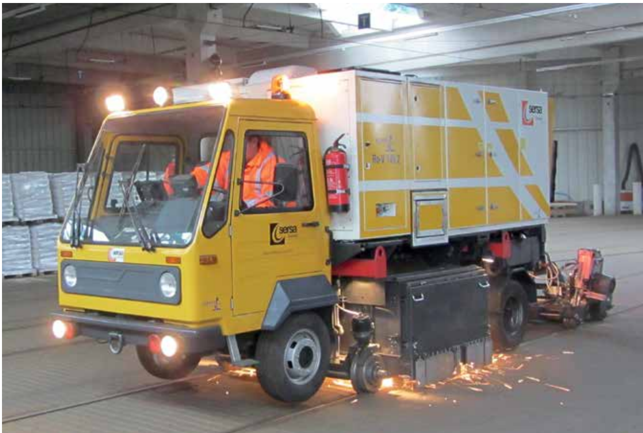
The machine has been specifically designed for local transport enterprises. It has extremely low noise and dust emissions, and placing it on tracks and removing it again only takes a few minutes.
