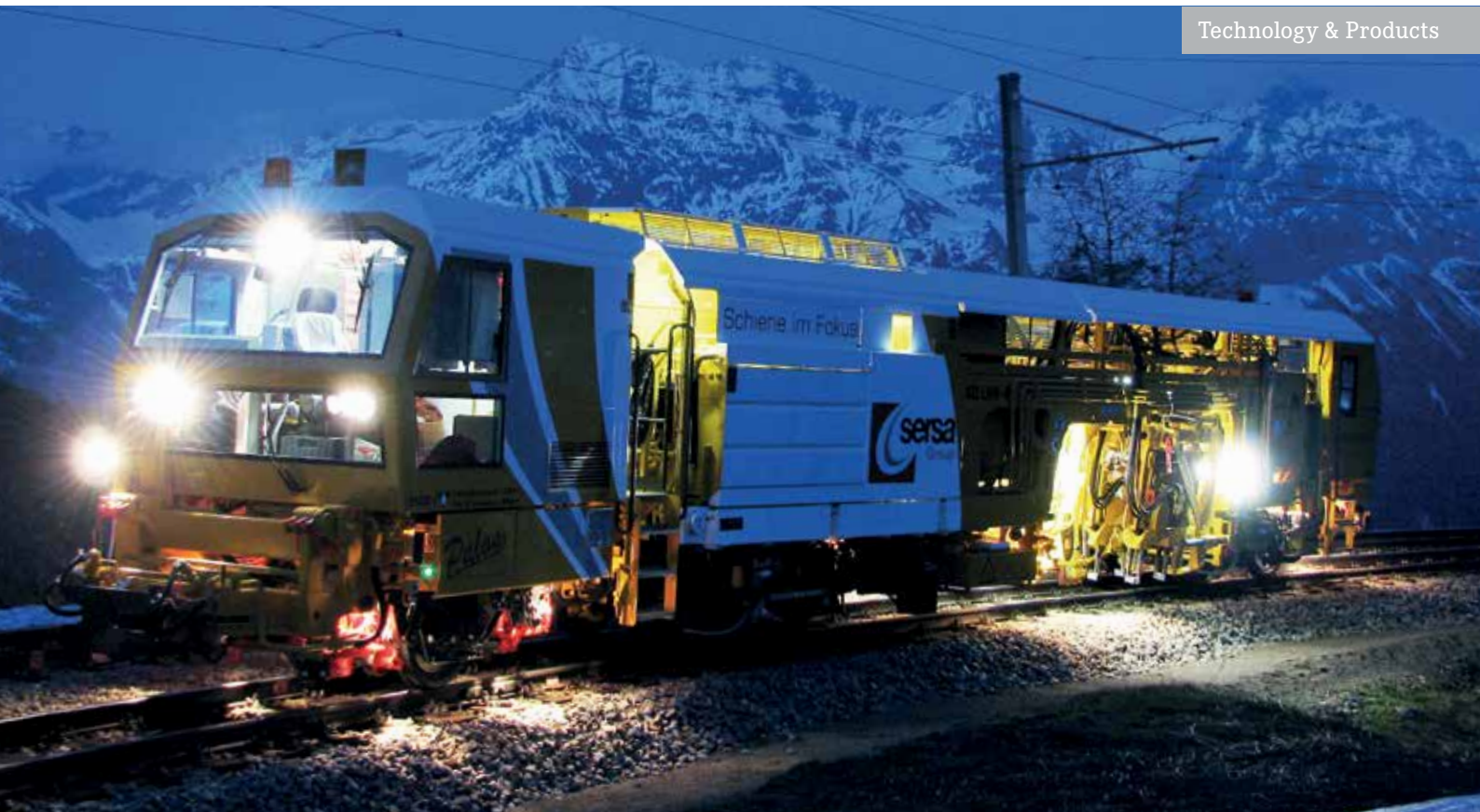
The tamping machine of Sersa Maschineller Gleisbau AG is able to collect network data.
