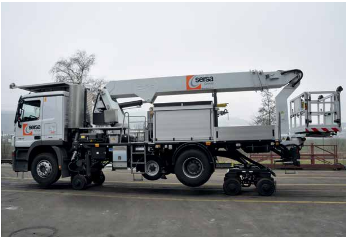
Mercedes Actros 1832, aerial platform and "SRT" track motion chassis.
