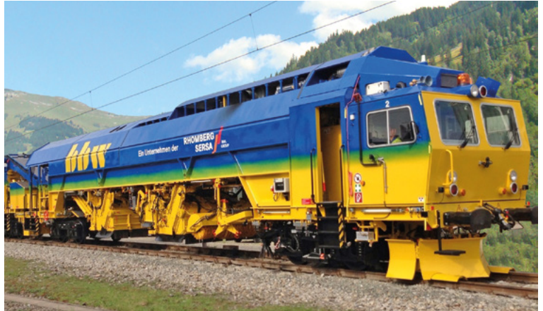
The new BDS 2000-4 ballast management system of BBW.
