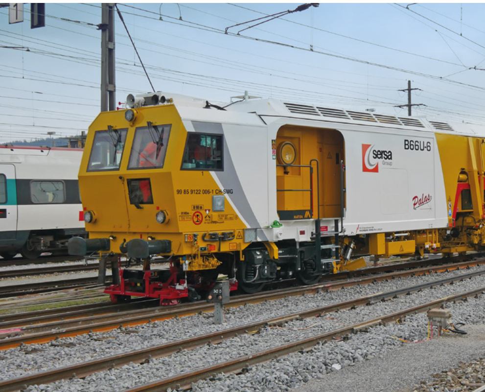
The "all-in-one" B66U-6 measures, tamps, compacts and levels - in one run.
