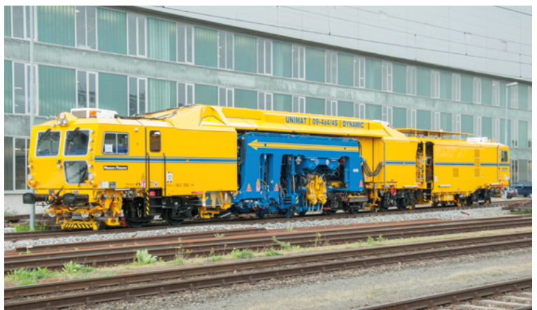
The new Unimat 09-4x4/4 S Dynamic tamping machine of JumboTec
