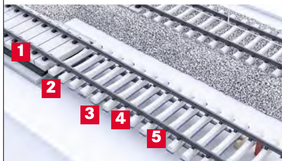
1 Slab track | 2 FF support & fixed support for V-TRAS 3 Elastomer (blue) | 4 Standard sleeper | 5 V-TRAS module
